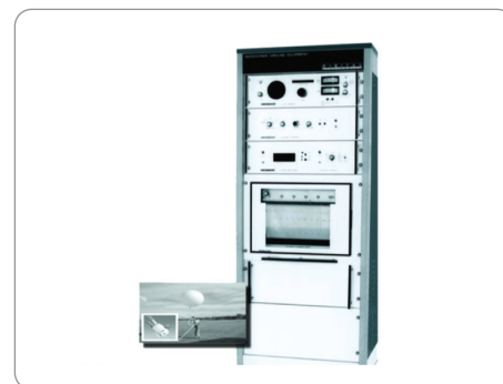
4 Radiosonde Ground Equipment
